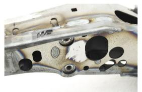
24. If the steering rack relocation needs to be Formula Drift legal, the tabs between the insert and lower control arm mount needs to be cut through. Use chisel to cut the tabs. NB! If the subframe does not have to be FD legal, then this is not necessary.
