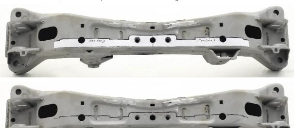
7. Place the masking tape along the cutting edge and cut the tape as shown in the picture. Check with the washer WFIS9\_ 106 if there are at least 3 mm gap between the mounting surface and the masking tape edge. Repeat the same on the orther side. Mark the cutting lines.
