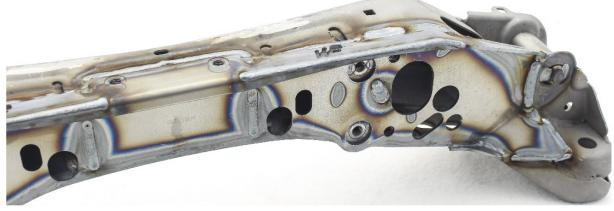
23. Grind flat the weld next to the steering rack mount.
