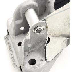
20. Mount the steering rack and make sure the insert is not bended.
