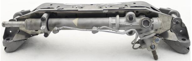
21. Tack weld the relocation insert. If the stock control arm mount is away from the rack relocation surface then clamp them together while tack welding.
