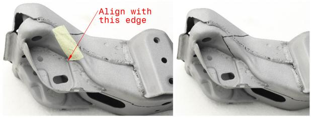
12. Place the masking tape along the edge to the mounting surface. Mark the cutting line.
