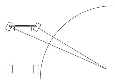
In drifting turning the wheels to the same side the instant center is actually on other side of the car, so from geometrical perspective reverse Ackermann is needed.
