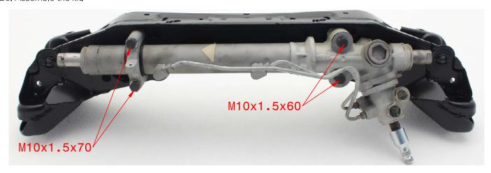
27. Use the small bushings between subframe brace and fixtures on body.
