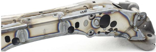
23. Grind flat the weld next to the steering rack mount.
