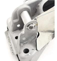
20. Mount the steering rack and make sure the insert is not bended.
